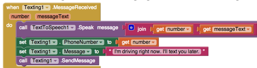
Fig. 1: An App Inventor program that speaks and responds to a text message.
